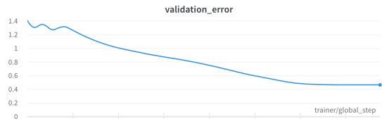
(b) Additional experiments show that the second peak is followed by a long period of monotonical decrease in validation loss.
